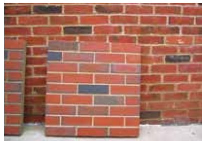
The precaster fabricated 1,758 panels using a blend of five brick colors. In all, more than 1 million pieces of brick were embedded into the panels. Photos: Gate Precast Co.
